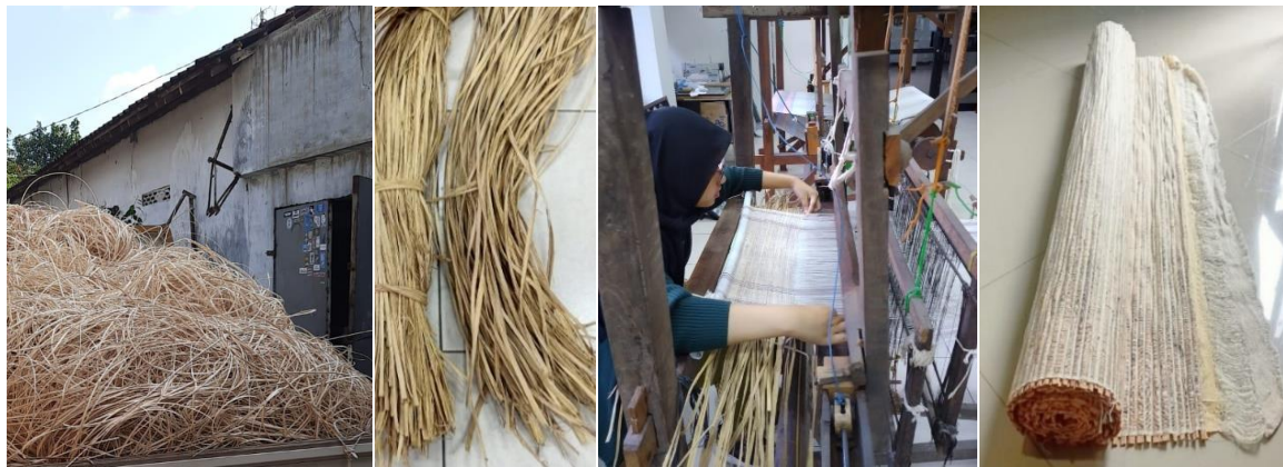
Fig. 2. From left to right: (a) Waste from rattan splitting process; (b) Waste processed into rattan fiber strips; (c) Weaving process; (d) Roll of woven rattan fiber strip sheets, 1 meter wide.
