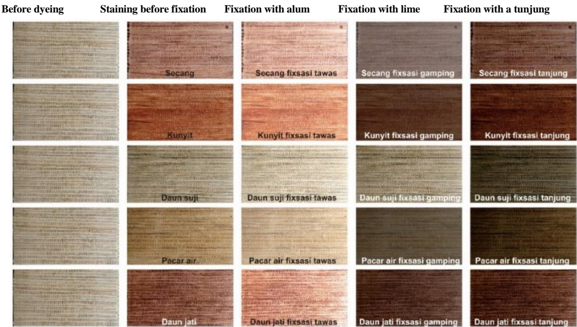
Fig. 3. The results of natural dyeing on woven rattan fiber strip sheets using secang , turmeric, pandan leaves, indigo, and teak leaves with the fixatives alum, chalk, and teak fixing
