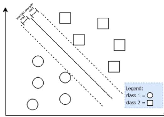
Fig. 1. Illustration of SVM classification based on hyperplane for two classes
