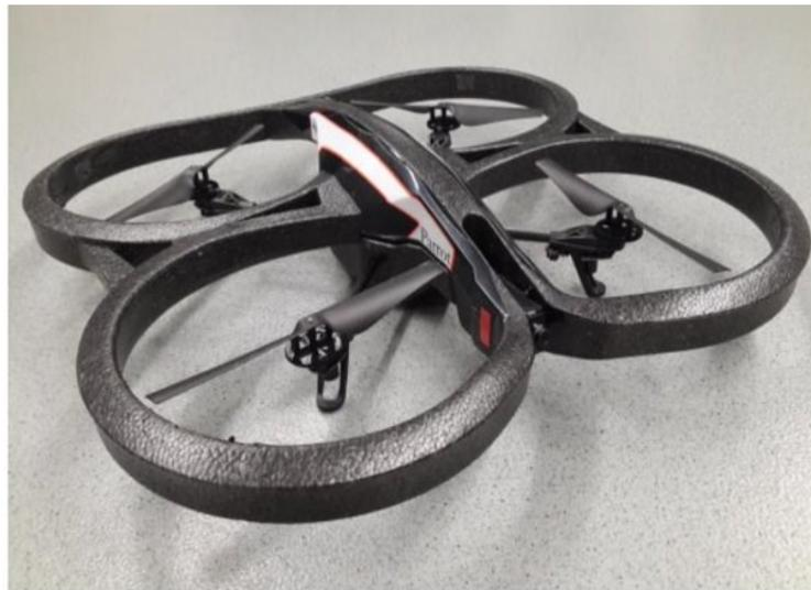
Fig. 3. Parrot AR Drone 2.0 with indoor hull
