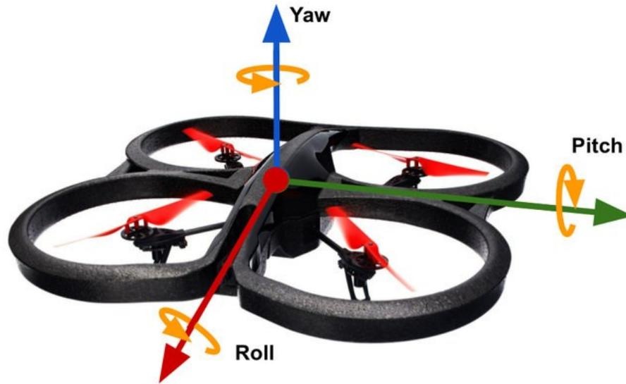
Fig. 2. Rotor-propeller connection and rotational movements of the quadrotor UAV
