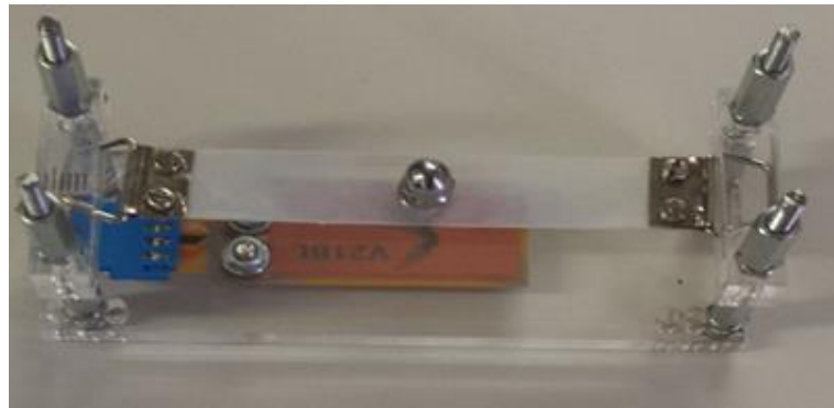
Fig. 3. Experimental Setup for the energy harvesting from vibration using piezoelectric materials
