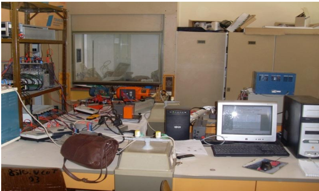
Fig. 9. Experimental setup for the proposed neural-fuzzy MRAS control of the IM
