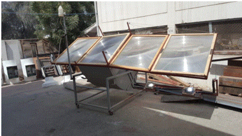
Fig. 14. Four fresnel lenses are arranged in series in the field location, Sharjah UAE
