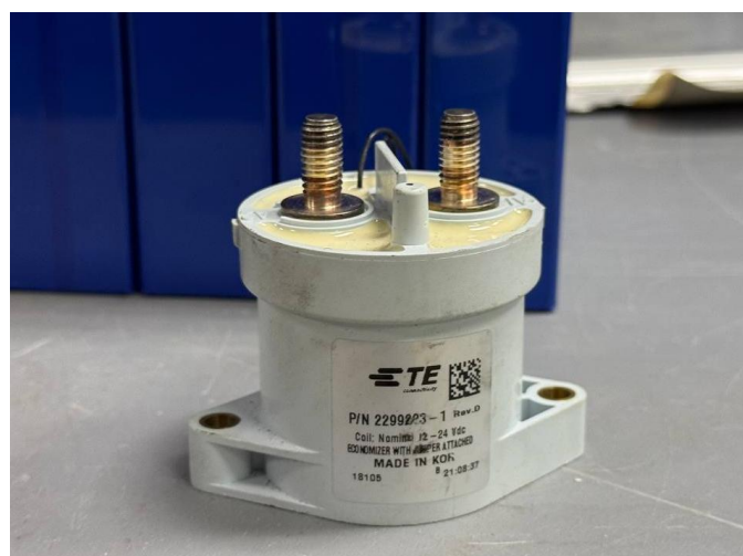
Fig. 17. A contactor can carry bigger current than a typical relay
