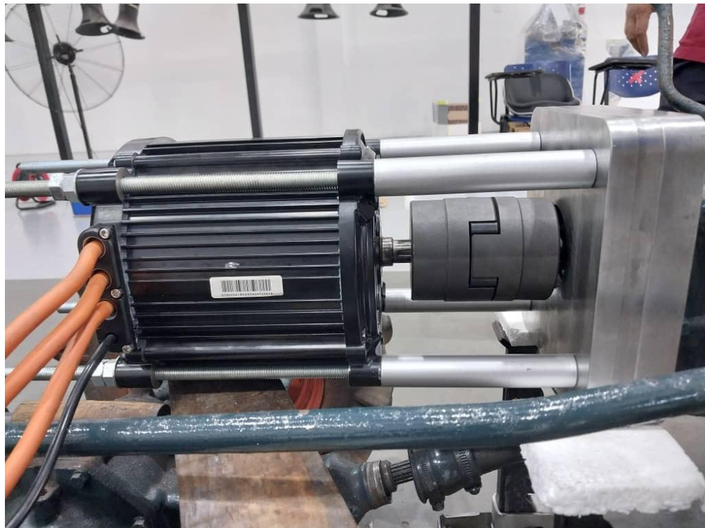
Fig. 33. Support bracket for the electric motor mount and the coupler
