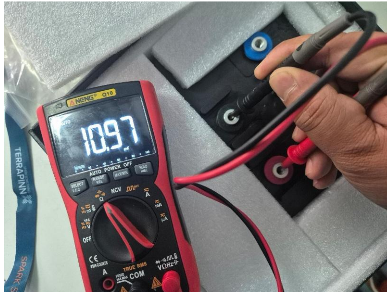
Fig. 36. Measured capacitance across the motor controller
