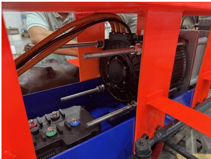
Fig. 31. Electric motor and motor controller underneath the structure
