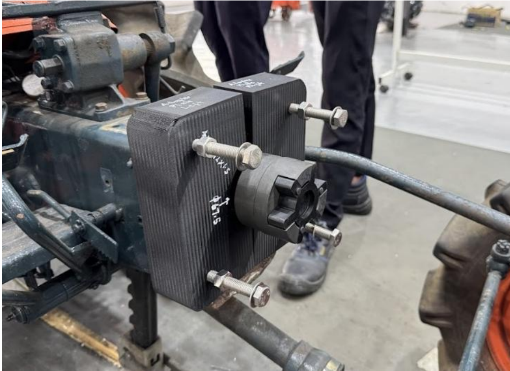
Fig. 32. The flexible jaw coupler with a 3D printed support bracket
