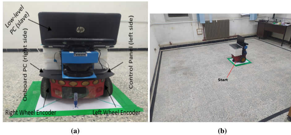
Fig. 11. Environmental modelling (a) Adapt Mobilerobots Pioneer 3-Dx, (b) Real environment of mobile robot
