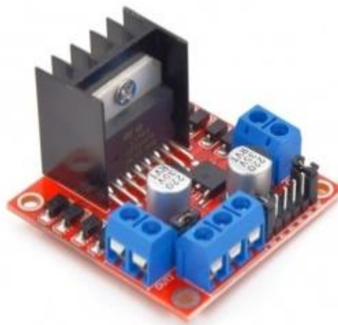
Fig. 4. L298N dual H-bridge driver module
