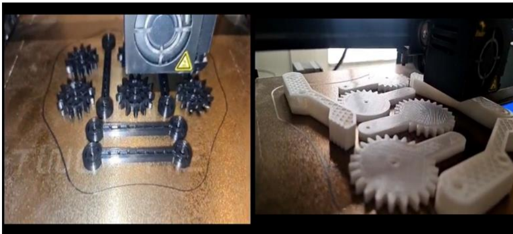
Fig. 10. Printing the small parts of the end-effector
