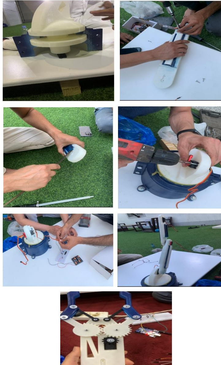
Fig. 12. Some taken photos during the assembly process of the developed 5-DOF robotic manipulator
