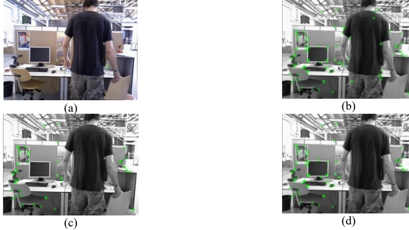
Fig. 9. Comparison of dynamic feature suppression effects (a). RGB, (b). ROB-SLAM2, (c). Epipolar geometric constraints, (d). Ours
