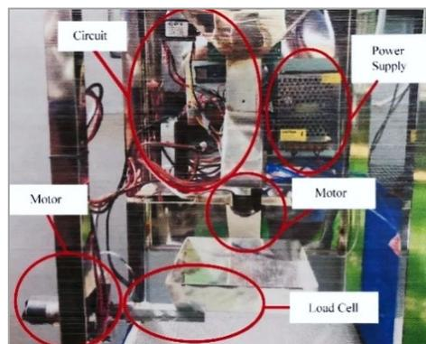
**Fig. 13.** Connection of components to the microcontroller
