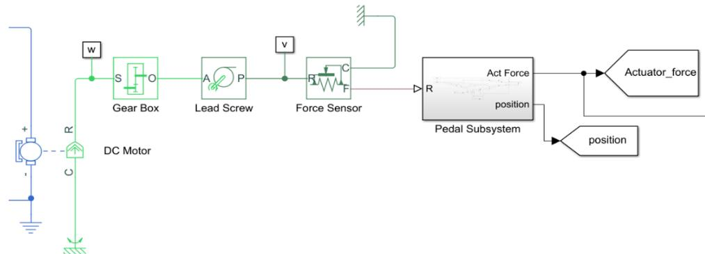
Fig. 4. Electrical actuator design in Matlab-Simulink
