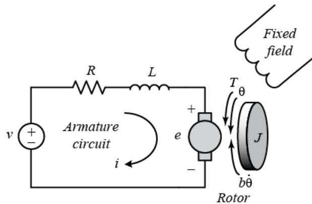
Fig. 2. Schematic of a DC motor system
