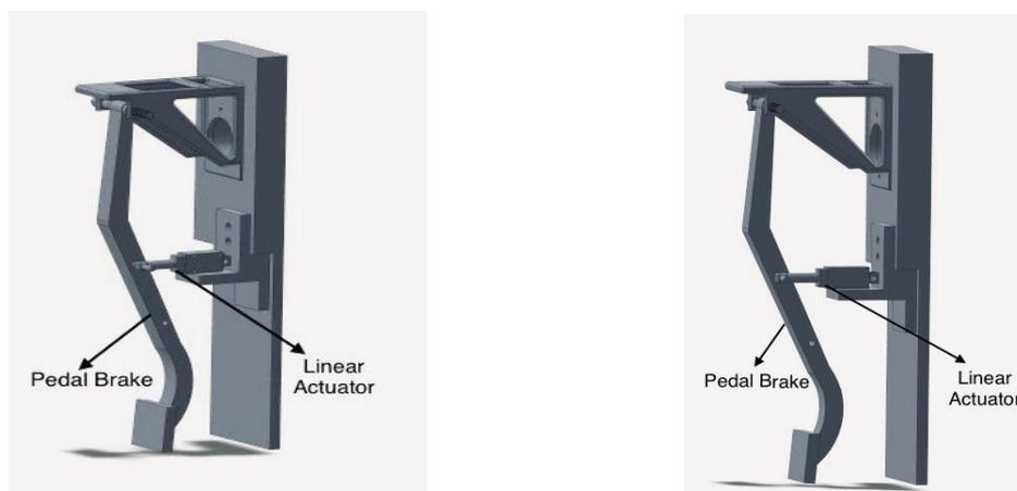
Fig. 1. Proposed design pedal brake with linear actuator
