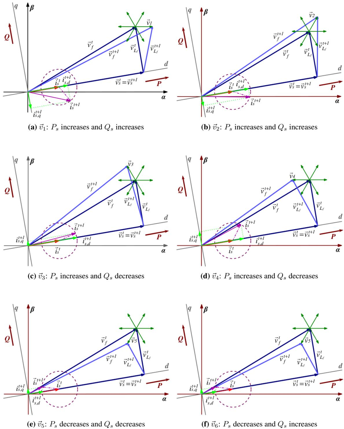
**Fig. 9.** Effect of Inverter Output Vector on Reactive and Active Powers
