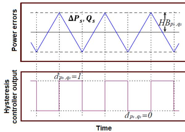
Fig. 7. Two-Level Hysteresis Power Comparator
