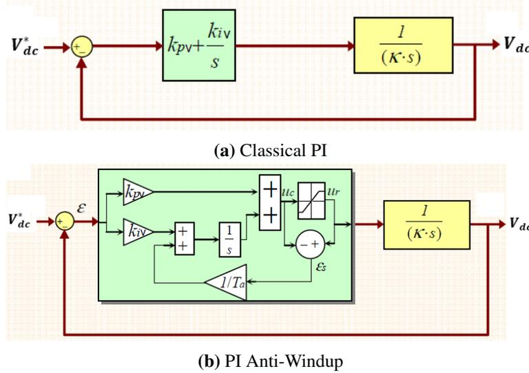
Fig. 5. Diagram of DC-Bus Voltage Regulation
