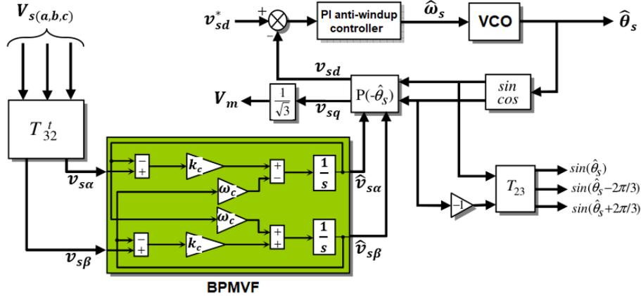
Fig. 4. Diagram of the New Structure of PLL with the BPMVF
