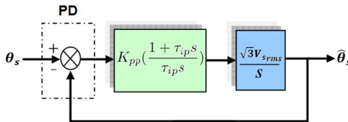
Fig. 3. Simplified Diagram of the PLL
