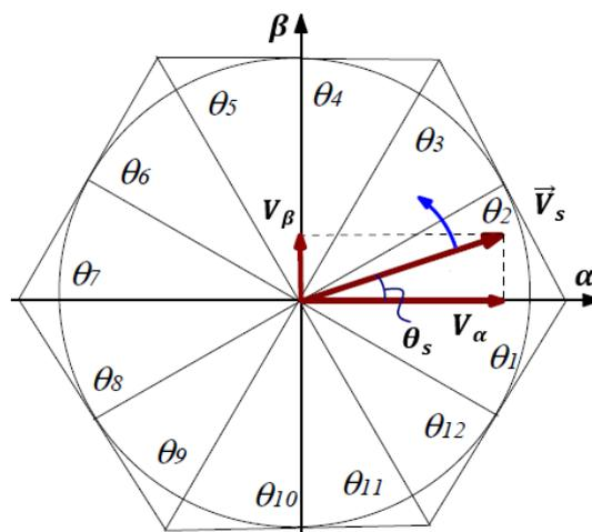
**Fig. 8.** Voltage Vector Representation in the Space Vector
