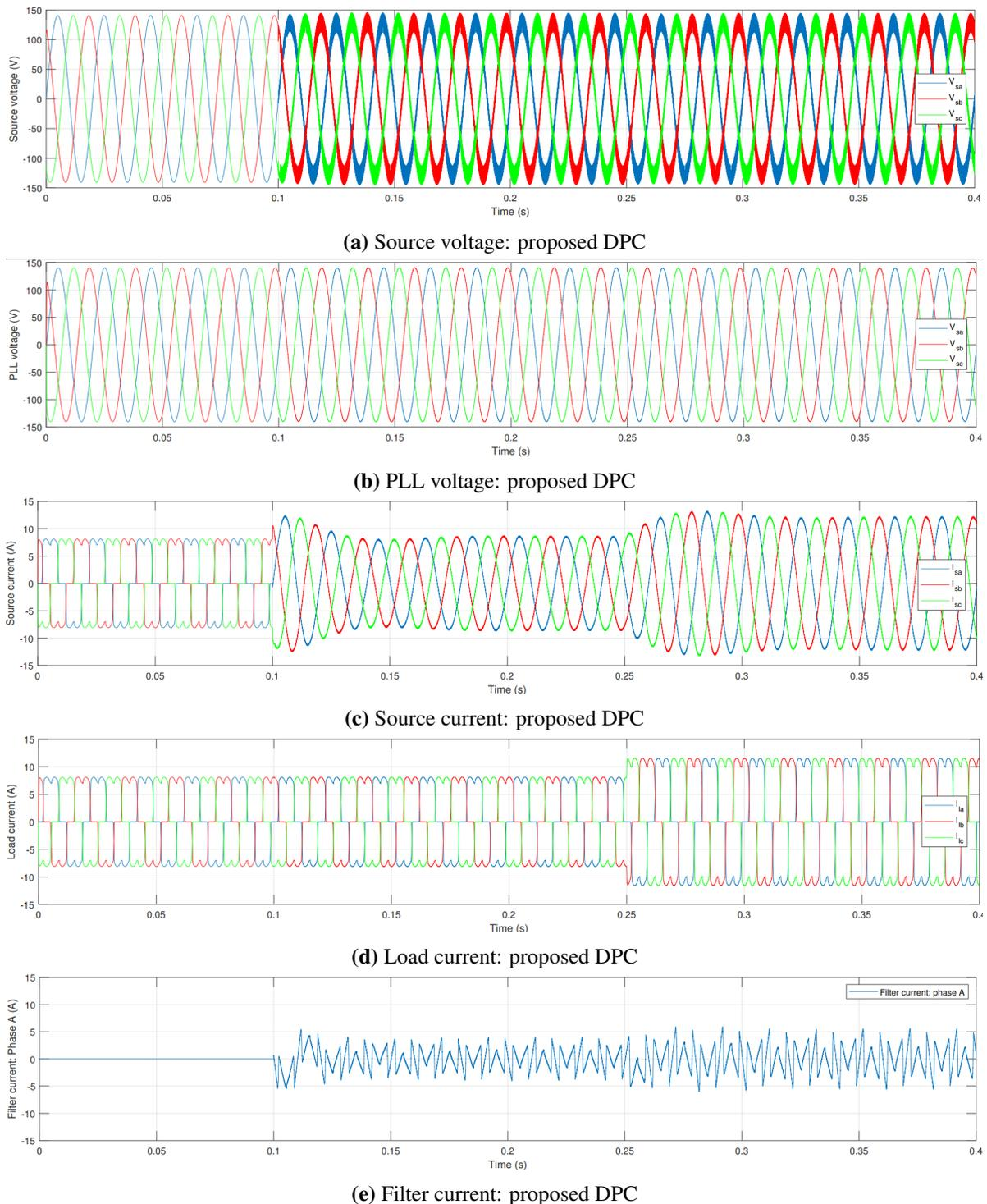
**Fig. 10.** Simulation Results of the Transient when Closing the SAPF at  $t=0.1$ s for a Variable Non-Linear Load
