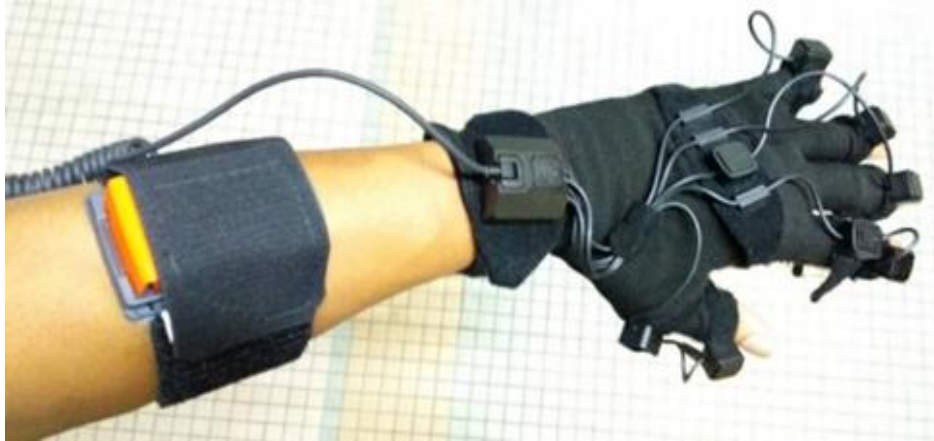
Fig. 7. Healthy upper limb with perception neuron glove and IMU from Xsens
