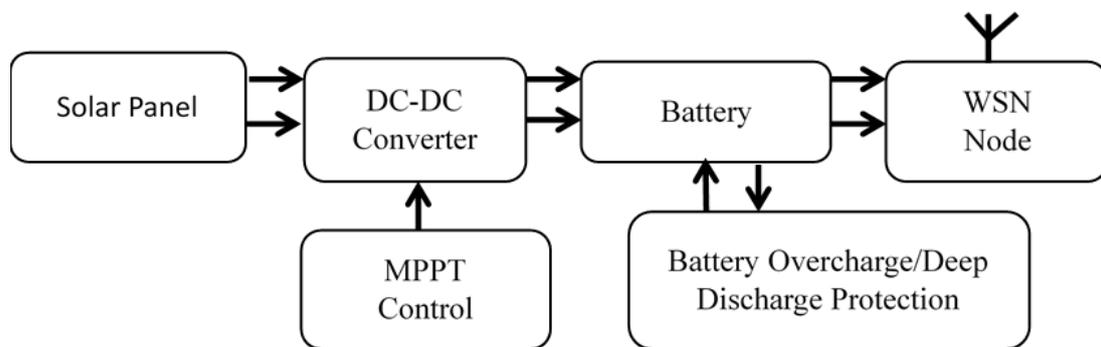
Fig. 4. A block diagram of solar energy harvesting mechanism [41]
