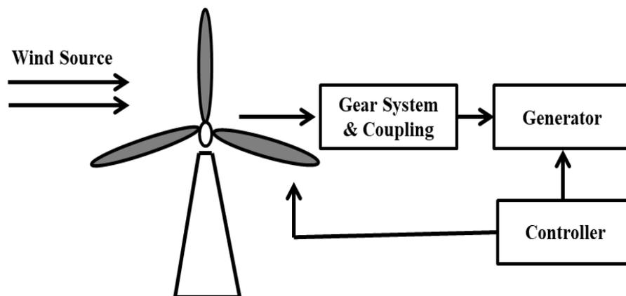
Fig. 5. Wind energy harvesting mechanism [43]
